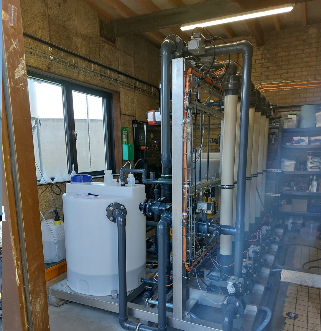
Total membrane area 90 m 2 Hollow fiber dNF40 membrane by NX Filtration Freedom in process conditions/staging Automated hydraulic and chemical cleaning Only screen filter as pre-treatment
